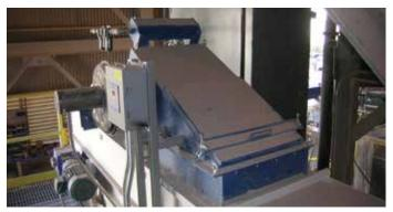
CPV-2 - Weigh belt feeder with limestone dust 800 cfm (1,359 m<sup>3</sup>/h)
