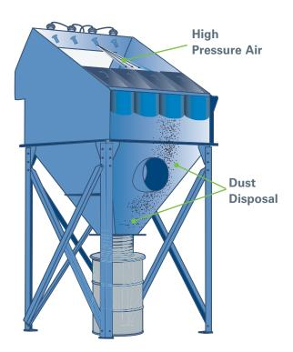
**FILTER CLEANING OPERATION** FOR CPC-3 THROUGH CPC-48 MODELS
