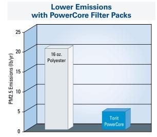
Independent lab results obtained using ASTM D6830-02 per EPA PM 2.5 performance verification. Annual emissions calculated assuming 14.400 cfm (24.461 m<sup>3</sup>/h) airflow rate, 265 working days per year, and two shifts per day. Field measurements may vary due to differences in dust contaminant and sensitivity of measurement equipment.
