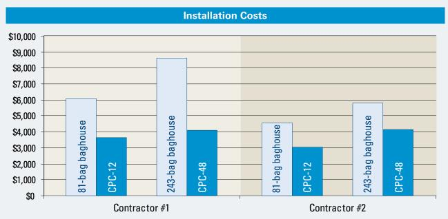
The Torit PowerCore system arrives mostly assembled, so installation is faster and easier, Installation costs are reduced 30-50% due to lighter weight, less crane time, and pre-assembly. The filter packs come pre-installed in the collector, so there are no bags or cages to install separately.
